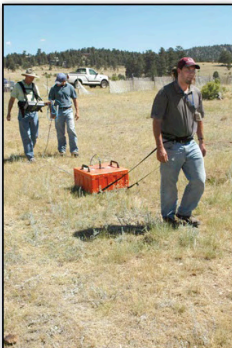
The soil scientists working with the Ground Penetrating Radar.
