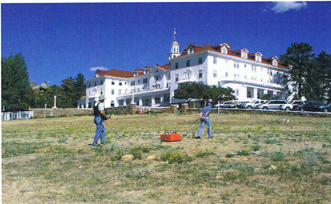
Photo 3. A GPR survey is being conducted at the Stanley Hotel, Estes Park, CO. Andy Steinert, MLRA Soil Survey Leader (USDA/NRCS) pulls the 200 MHz antenna at a consistent pace across the survey area while Wes Tuttle, Soil Scientist (Geophysical), (USDA-NRCS-NSSC) reviews ground penetrating radar (GPR) survey data. GPR surveys usually require at least two people, one person to pull the antenna and another person to collect and record the data.
