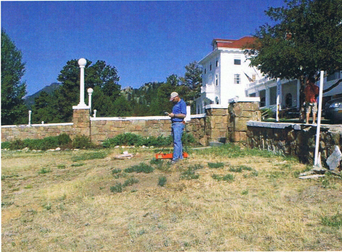
Photo. 1 Wes Tuttle, Soil Scientist (Geophysical), USDA/NRCS/NSSC prepares for an EMI survey near the Stanley Hotel, Estes Park, CO. The survey is being conducted with the EM38 meter, an Allegro field computer and a Holux GPS receiver. This data collection system allows for the collection of much larger data sets in combination with geo-referencing of apparent conductivity measurements.
